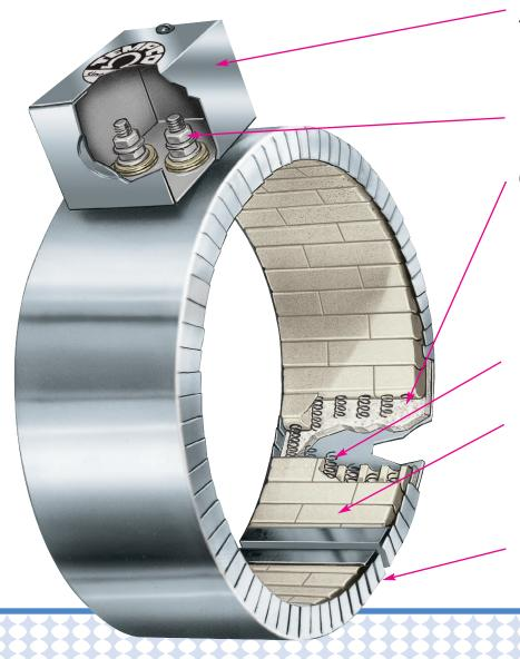
General purpose terminal box offers excellent protection to exposed terminals. To simplify electrical wiring, the box has a 1/2" trade size knockout (actual dia. 7/8") that will accept standard conduit or flexible armor cable connectors.
