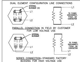
**DUAL VOLTAGE HEATER NOTE;** HEATERS WITH TWO ELEMENTS MAY BE USED AS DUAL VOLTAGE HEATERS. WHEN WIRED IN PARALLEL, FOR LOW VOLTAGE USE, ELEMENT VOLTAGE EQUALS LINE VOLTAGE. WHEN WIRED IN SERIES, FOR HIGH VOLTAGE USE,
